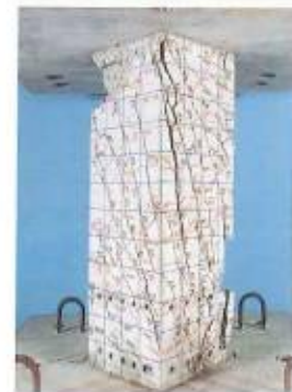
F_c = 60 \text{ N/mm}^2 SD 490 rebar axial force ratio (N/No) = -0.7 ~ +0.5 loading direction: 45^\circ
